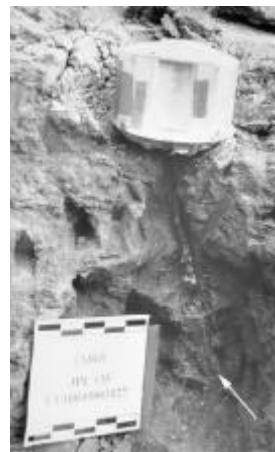
Cutaway view of test microprobe after it was fired into hard, frozen ground by an air gun.
