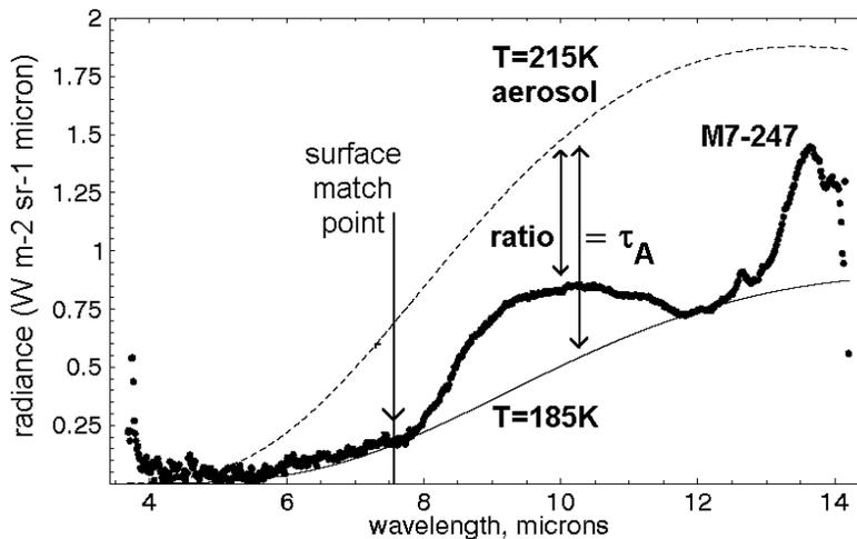
**Fig. 2: Conversion of night spectrum to apparent transmission.** This shows a typical IRS spectrum measured of Mars at night. The spectrum is converted to apparent transmission as described above. However, in night spectra, the background (surface, solid line) is colder than the zero reference line (dashed). The zero reference line gives the value that would be seen if the aerosol transmission is zero.
